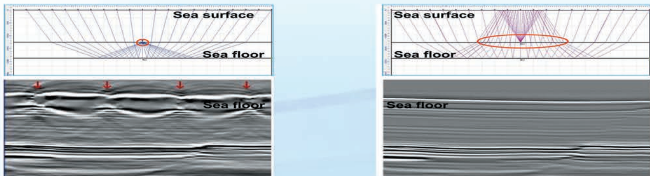
Illumination of up–going wave PSTM (left) vs. down–going wave mirror PSTM (right)
