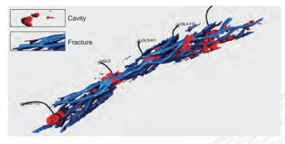
3D carving visualization diagram of a fault controlled fractured-vuggy unit
