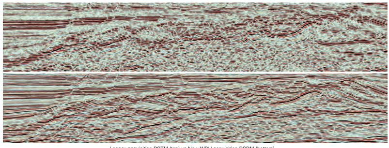
Legacy acquisition PSTM (top) vs New WBH acquisition PSDM (bottom)
