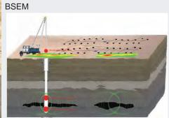
Schematic diagram of BSEM field operation
