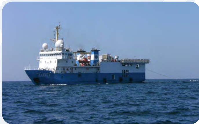
DONG FANG KAN TAN NO1 Seal 428 recording system 1 × 12km Solid streamer Advanced INS
