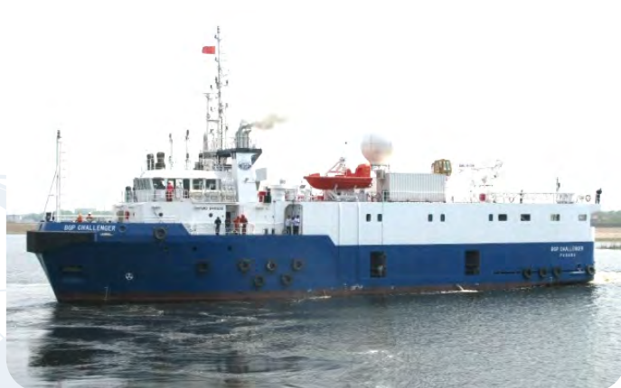
BGP Challenger Seal 428 recording system 2 × 6 km Solid streamer Advanced INS
