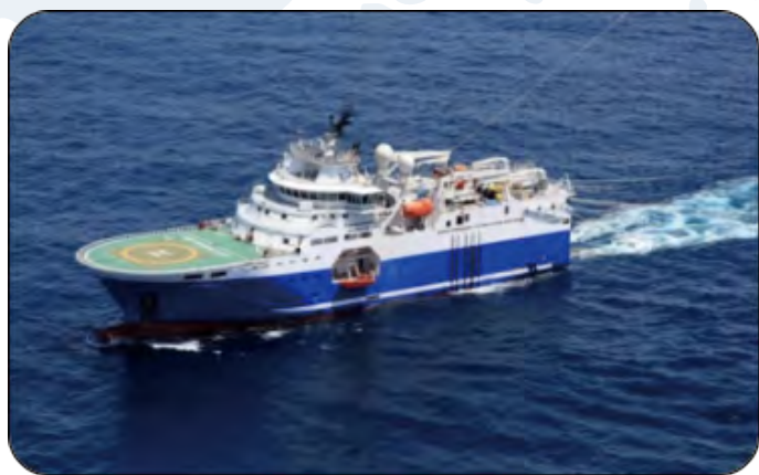
BGP Prospector Seal 428 recording system 12 × 8km Solid streamer Steerable source Advanced INS
