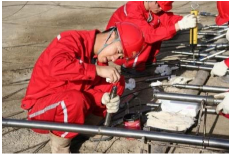
3C geophone routine maintenance
