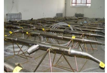
GeoWave 3C down-hole receivers 32 levels 20,000psi, 180 °C
