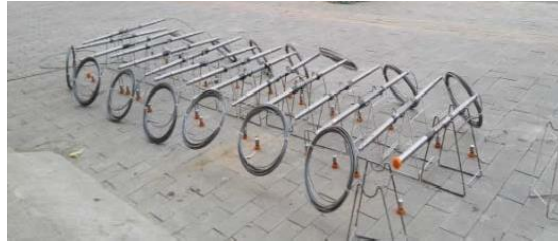
Model: Geochain SlimTM (3-Component) Max outside diameter: 43mm (1" 11/16)
