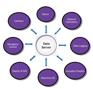
Dolphin is an integrated navigation and control system designed to meet the demanding needs and challenging environments of multi-vessel distributed operations such as ocean bottom cable and shallow water seismic operations. Dolphin delivers a unique combination of centralization, data management, advanced positioning techniques, and flexible configuration. The system not only improves the acquisition quality and the production management, but also reduces the cost of operation.
