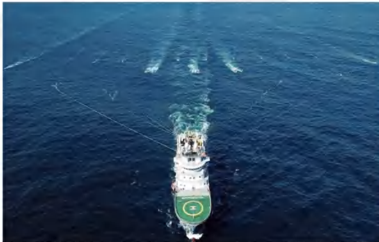
Towed streamer acquisition with 12 x 8km cables and wide-towing triple source
