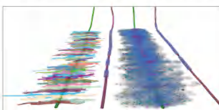
Continuous fracture network
