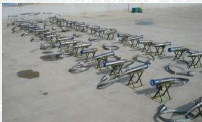
Model: MaxiWave (3-Component) Pressure rating: 1200 bars (17400psi) Temperature rating: 135°C(275°F)operating
