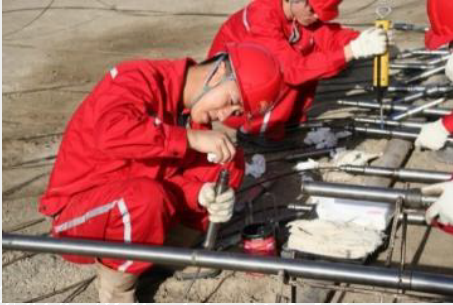
3C geophone routine maintenance
