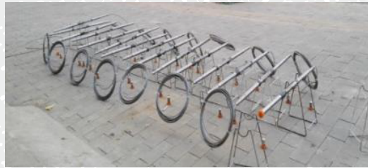
Model: Geochain SlimTM (3-Component) Max outside diameter: 43mm (1"11/16)
