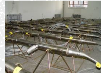
GeoWave 3C down-hole receivers 32 levels 20,000psi, 180 °C
